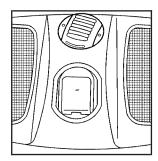
To express-open the sunroof glass panel and sunshade, press the switch rearward and release it. To stop the sunroof before it is completely open, press the switch rearward again. The sunshade cannot be closed with the sunroof open. To close the sunroof, press forward on the switch until it stops. The sunshade must be manually closed.
